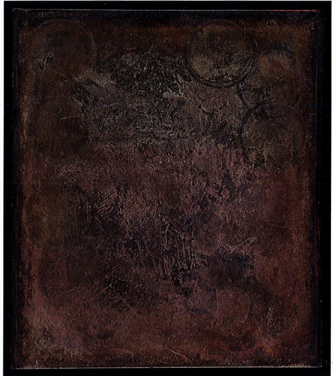
An optical image of a daguerreotype. Evidence of localized electro-cleaning attempts is visible as circular spots in the top left and right corners.
